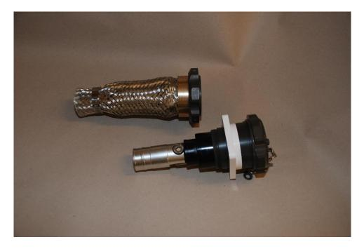
The braided shielded style receptacle is installed into the panel with the braided shield removed. The braided shield retaining ring is LEFT hand threaded and the braided shield and retaining ring assembly are removed by unscrewing to the right. The receptacle is installed with the gasket between flange and the panel wall.
